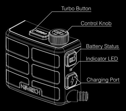
**Control Knob -** Turn to switch on, and then adjust the power of the fan up or down.
